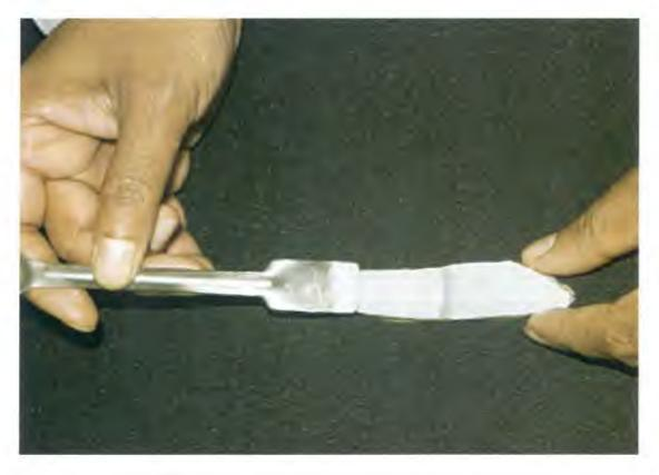
Fig. 9.198 Applying the slip prepared in the laboratory on the stone
