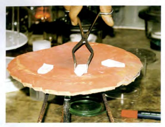
Fig. 9.199 Heating treatment to the coating, using terracotta plate
